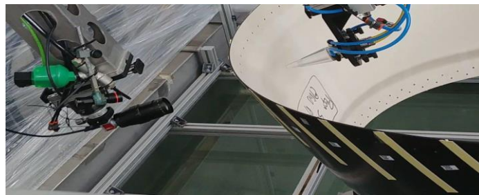
Figure 1. Industrial inspection held at Tecnitest with the high-speed camera attached on the lower side of the robotic arm.
