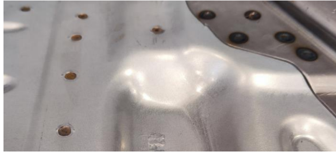
Figure 2. Different spot welds tested.
